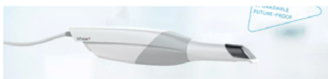
Figura 3 - Scanner intraoral trios 3shape (disponível em: https://www.3shape.com/en/scanners/trios ).
